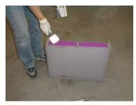
Using a clean and dry instrument, remove the sample of MULTI-MIX® media from below the top surface of the media bed in the module
